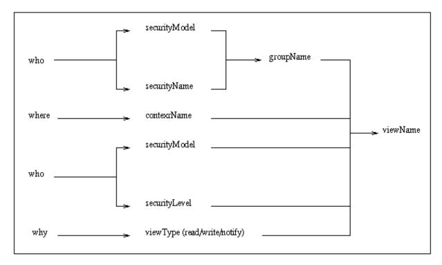
Figure 2.4: Overview of the mechanism of MIB selection
