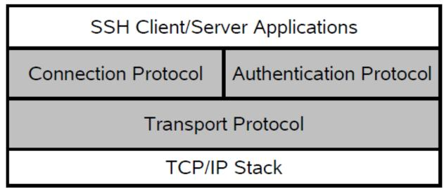
Figure 1.1: SSH Protocol Architecture
