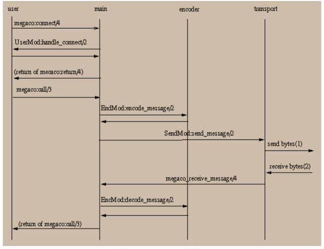
Figure 3.2: MG Startup Call Flow
