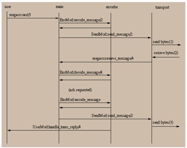
Figure 2.4: Message Call Flow (originating side)
